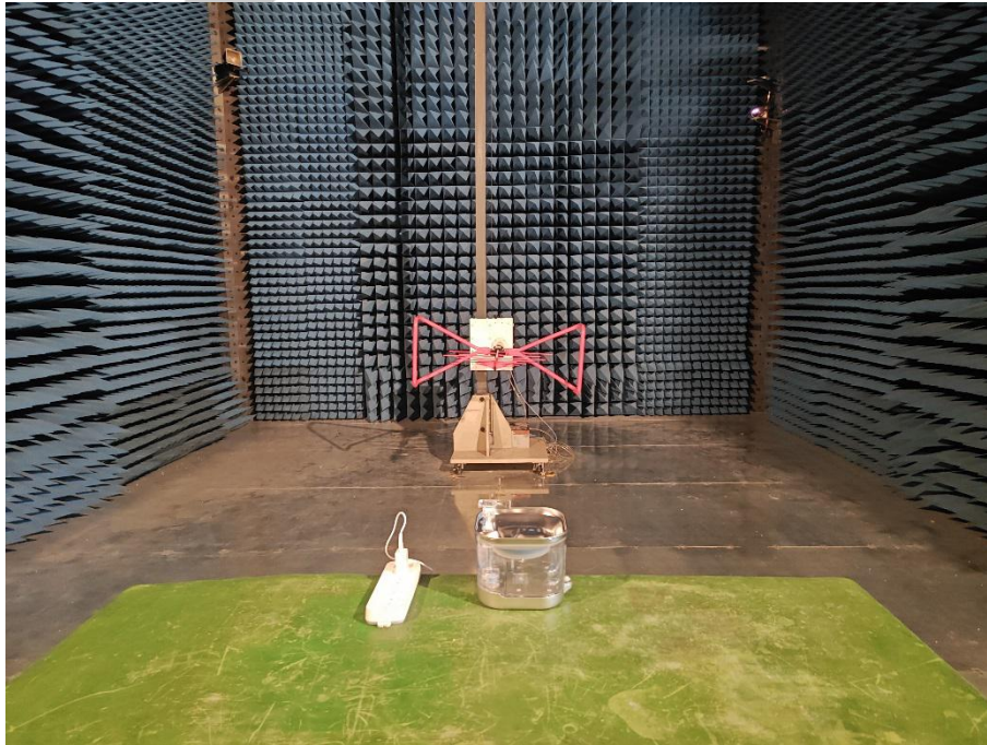
Radiated Measurement Photo
